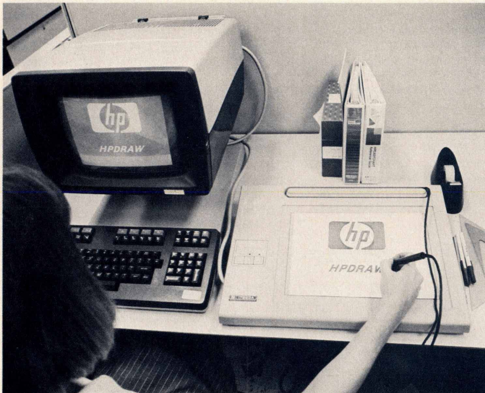
Fig. 7. When used with HPDRAW, the HP 17623A Graphics Tablet allows a user to create freehand drawings, digitize graphical data, and make menu selections.
